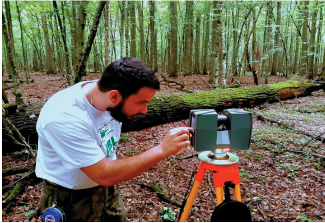
Figure 1. Terrestrial laser scanner parameterization (project LIFE + ForBioSensing PL; photographer A. Modzelewska)
