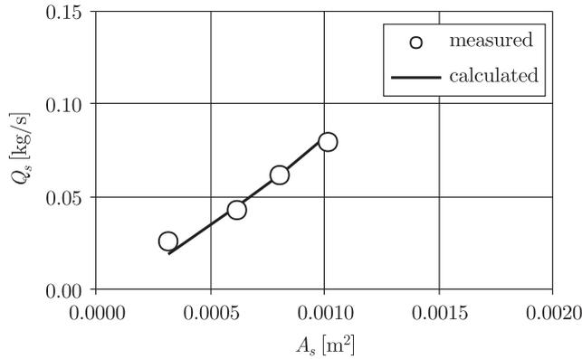
Figure 10. Mass flow rate,  $Q_s$ , as a function of outlet area,  $A_s$ , for a 66mm tube
