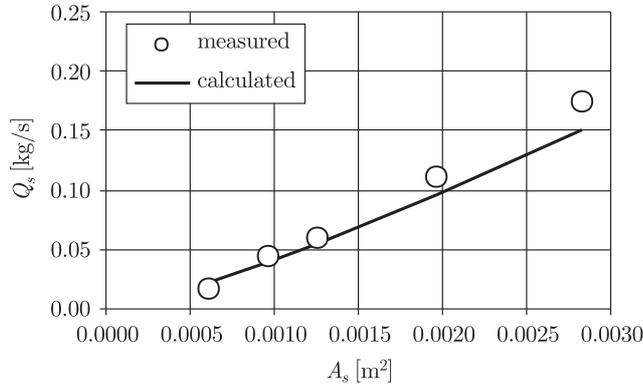
Figure 12. Mass flow rate,  $Q_s$ , as a function of outlet area,  $A_s$ , for a 110mm tube
