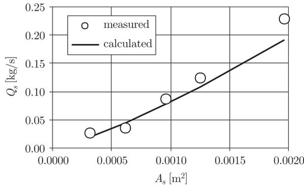
Figure 11. Mass flow rate,  $Q_s$ , as a function of outlet area,  $A_s$ , for a 92mm tube
