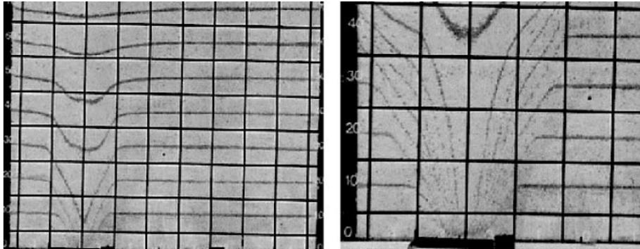
Figure 18. Mass flow in the model silo during eccentric discharge
