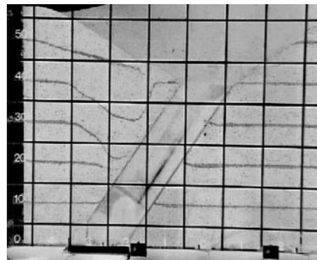
**Figure 17.** The tube is empty – the material flows through a side opening
