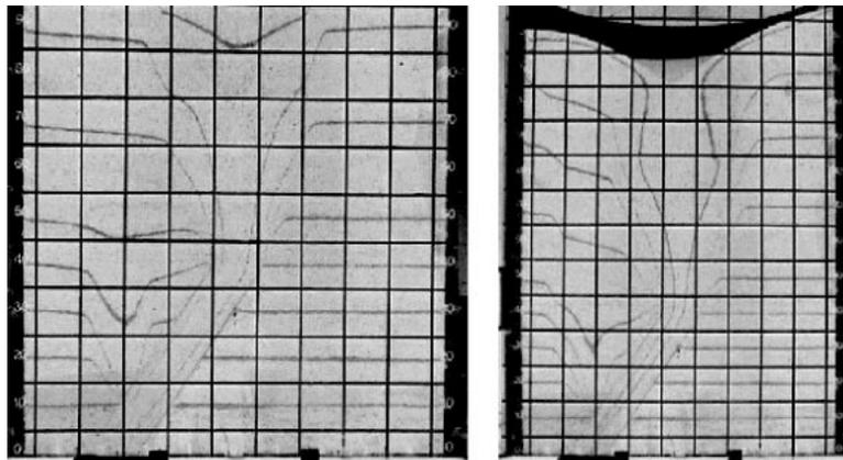
Figure 20. Emptying the silo through an improperly designed discharge device
