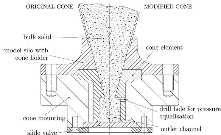
Figure 5. Cone design: left – original; right – modified
