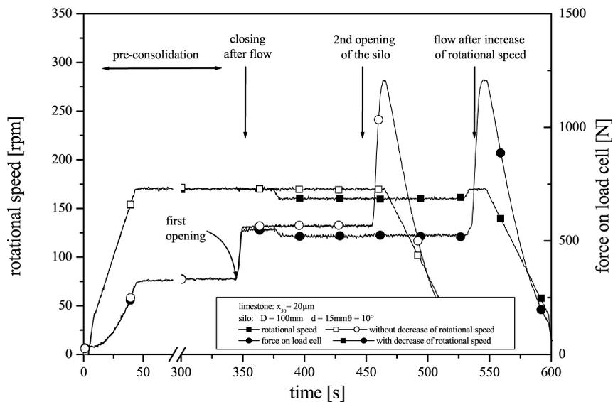
Figure 6. Test procedure to investigate the stress state after pre-consolidation (coarse limestone)
