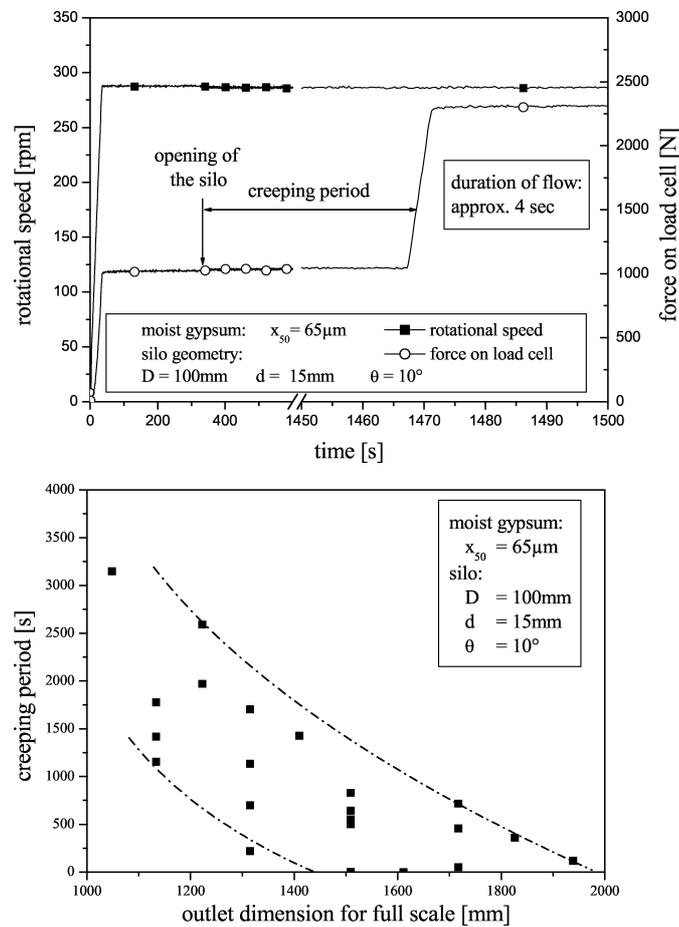
Figure 8. Top – testing procedure to investigate creeping of moist gypsum; bottom – creeping period versus the outlet dimension for full scale
