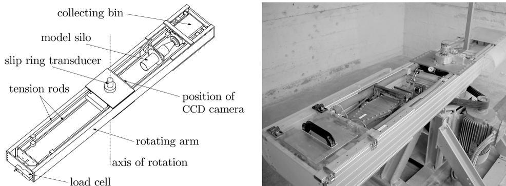
**Figure 2.** The silo centrifuge: left – a scheme with the model silo; right – a picture with the rotating arm turned 180°
