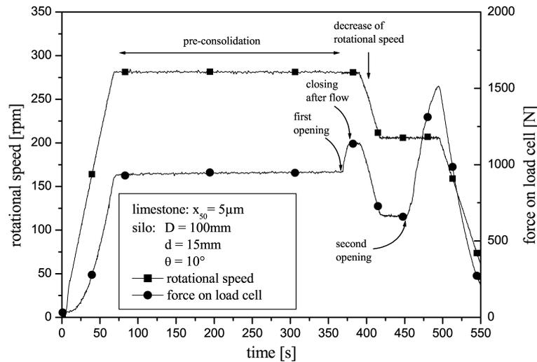
**Figure 7.** Test procedure to investigate the stress state after pre-consolidation (fine limestone)
