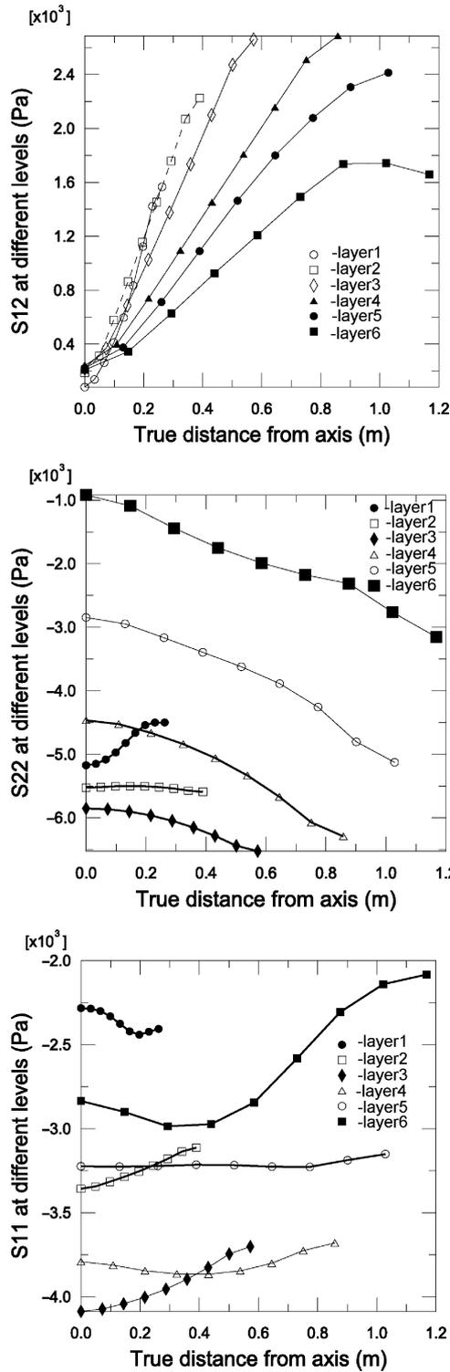
Figure 2. Stress developed along the middle lines of each layer during switch-on filling
