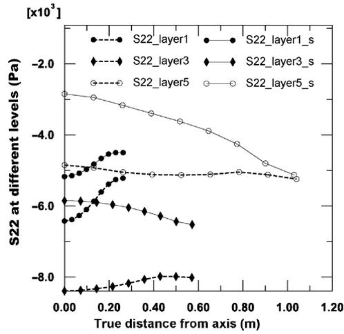
Figure 7. Comparison of stresses developed during various filling procedures
