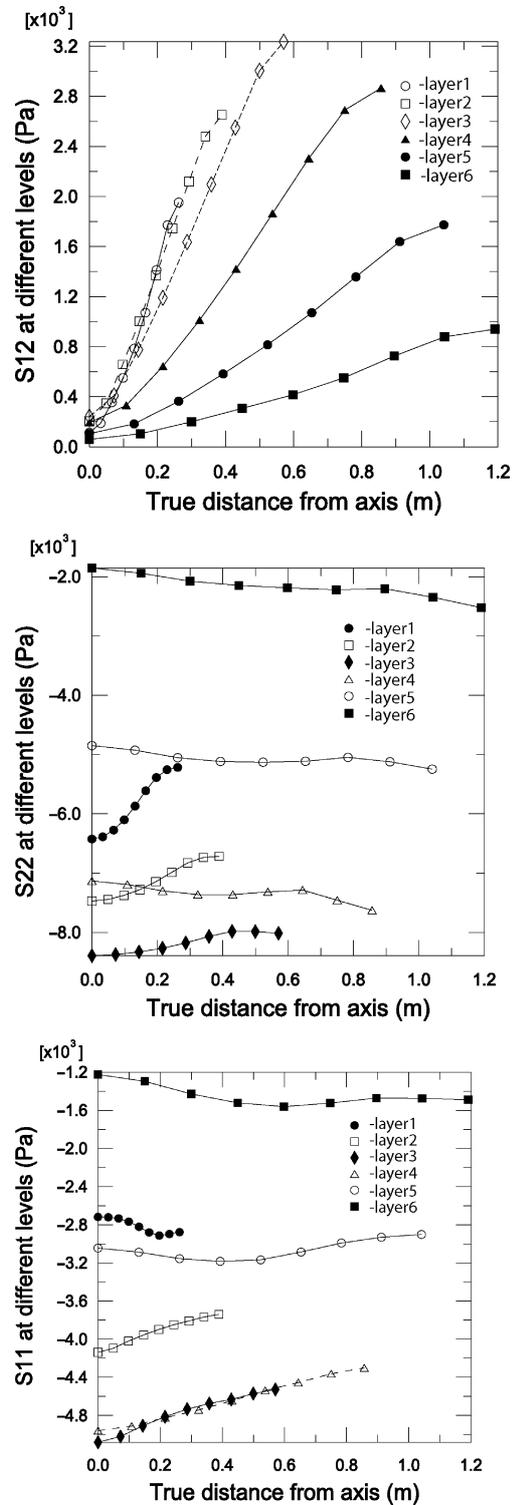
Figure 3. Stress developed along the middle lines of each layer during layer-by-layer filling
