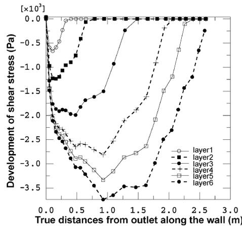
Figure 5. Development of friction stress distributions along the hopper wall
