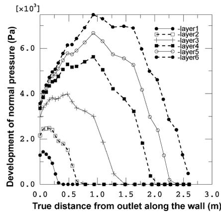
Figure 4. Development of normal pressures along the hopper wall
