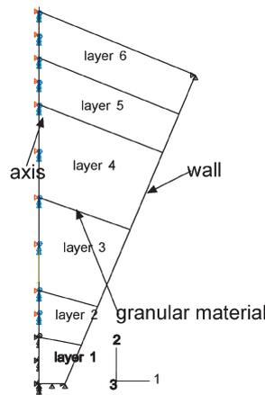
Figure 1. Hopper, granular material and boundary conditions
