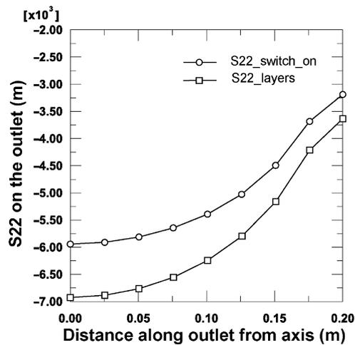
Figure 9. Vertical stresses at the outlet for the two filling processes
