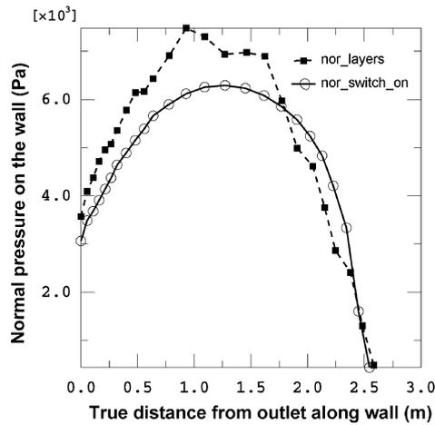
Figure 8. Loads along the wall for the two filling processes
